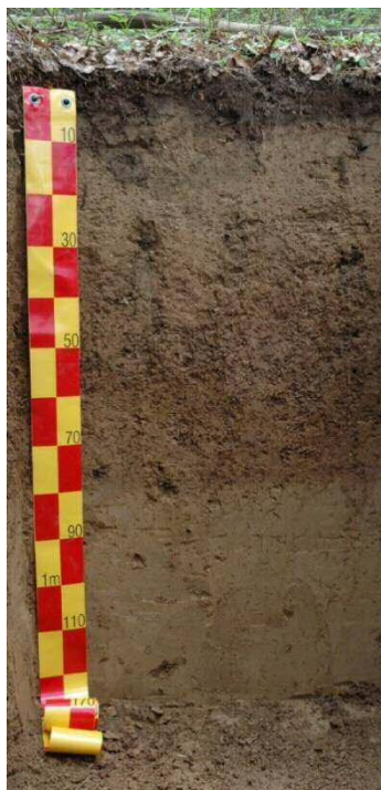
Figure 8.5: Ideal soil profile. Always take the photo perpendicular to the profile wall
