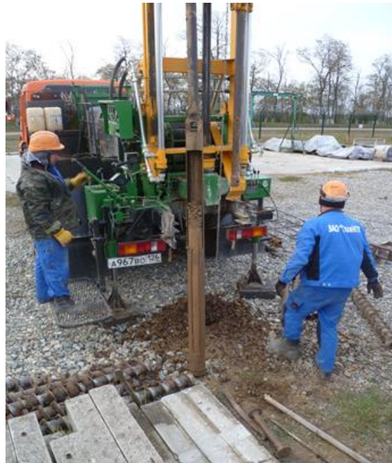
Photo 2. Sampling of monoliths with clay cutter SV-127
