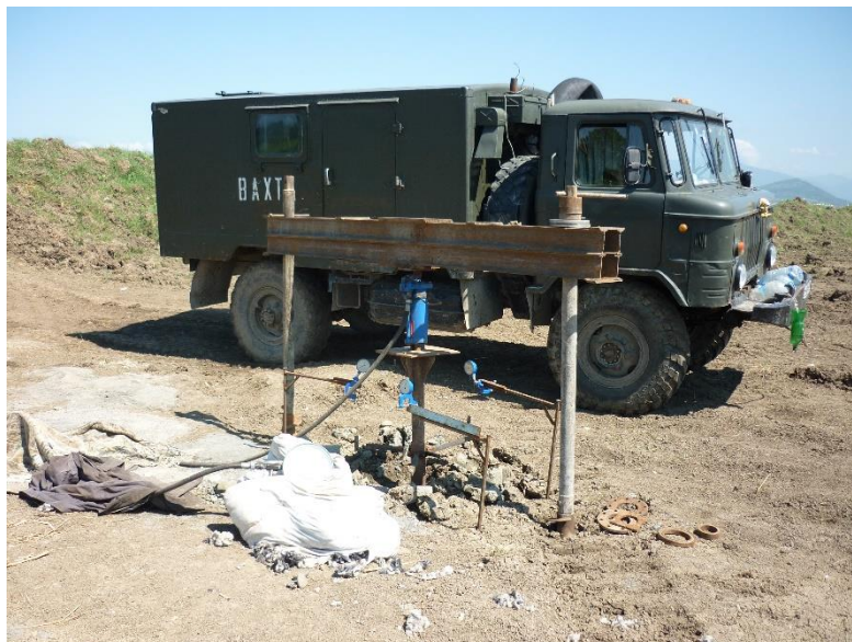
Photo 1. Screw test of static plate load of soils S=600 \text{ cm}^2
