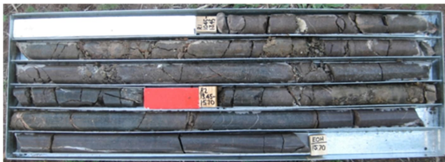
Figure 8-1: Example of Rock Core Photo with Core Loss
