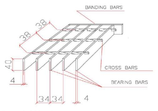
TYPE OF FORGE-WELDED GRATINGS EXAMPLE GRATING TYPE :SP 440-34/38-4
